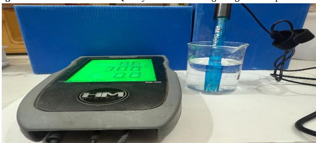
Image 4: Measurement of Water Quality Parameters Using a Digital Multiparameter Meter
