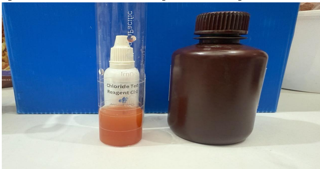
Image 7: Chloride Estimation in Water Using Chloride Test Reagent
