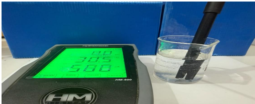
Image 5: Measurement of pH, Temperature and Electrical Conductivity of Water Using a Digital Multiparameter Meter
