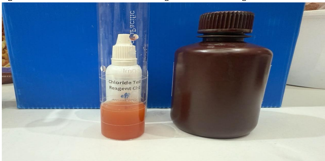
Image 7: Chloride Estimation in Water Using Chloride Test Reagent
